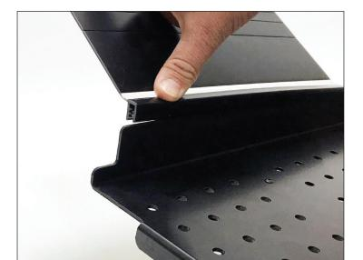
② On installed shelf, clip "U" channel of baffle to rear lip of shelf, with hinged fin of baffle facing rearwards. If installing on a shelf mounted to a Grid Assembly, ensure 10" fits between Grid Assembly uprights and contacts the rear wall of the case.
