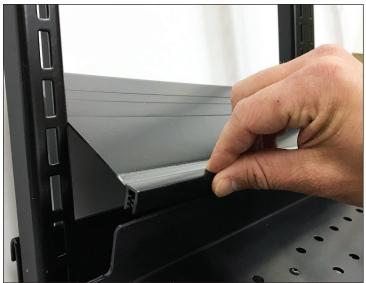
(3) Ensure baffle contacts rear wall of case (or comes within 1/8" of touching). Angle hinged fin of baffle downward if possible, to allow more case ventilation holes to provide air over the top of the shelf deck.
